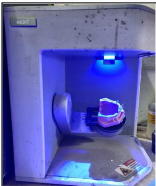
Fig. 25: Model with parallel pin being scanned
