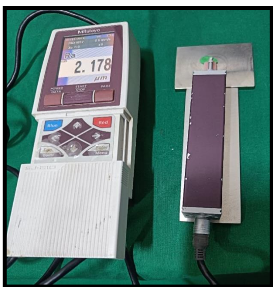
Figure 5: Surface roughness test by Profilometer
