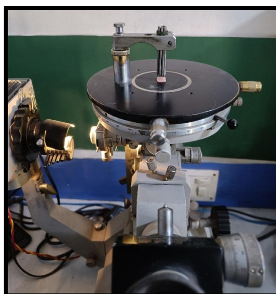
Figure 6: Microhardness test by Vicker's Microhardness tester
