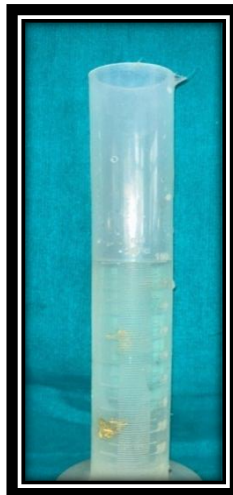
Figure 2: Immersion of post in 100ml of 24% Hydrogen Peroxide
