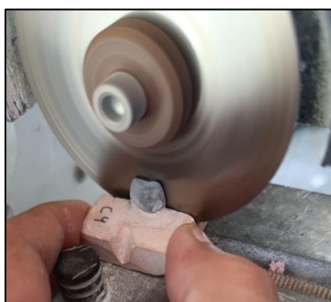
Fig 6: Sectioning of test specimens
