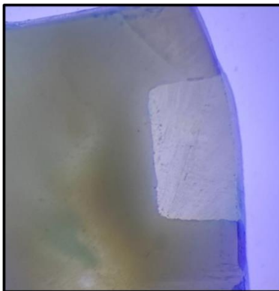
The Arrow 1 & 2 Shows no dye Penetration at Tooth Composite Interface (Occlusal wall & Gingival wall Score 0)
